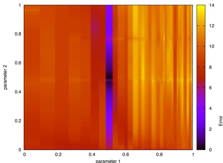
**Figure 3.4:** The error surface for the basic FM synthesizer. The colour indicates the distance in feature space from audio generated with that parameter setting to a reference feature generated with parameter settings 0.5, 0.5, hence the global minimum error at 0.5,0.5.
