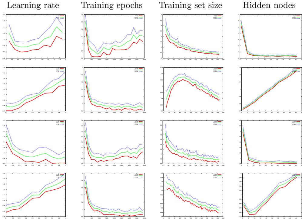
**Figure 3.10:** Neural network performance for the 4 synthesizers with varying network and training properties. Each row is for a different synthesizer: basic FM, complex FM, basic subtractive, and complex subtractive. Each graph shows the mean and standard deviation either side observed for 25 test runs. The test set error is plotted against each of the 4 network properties apart from the learning rate, where the training set error is used.
