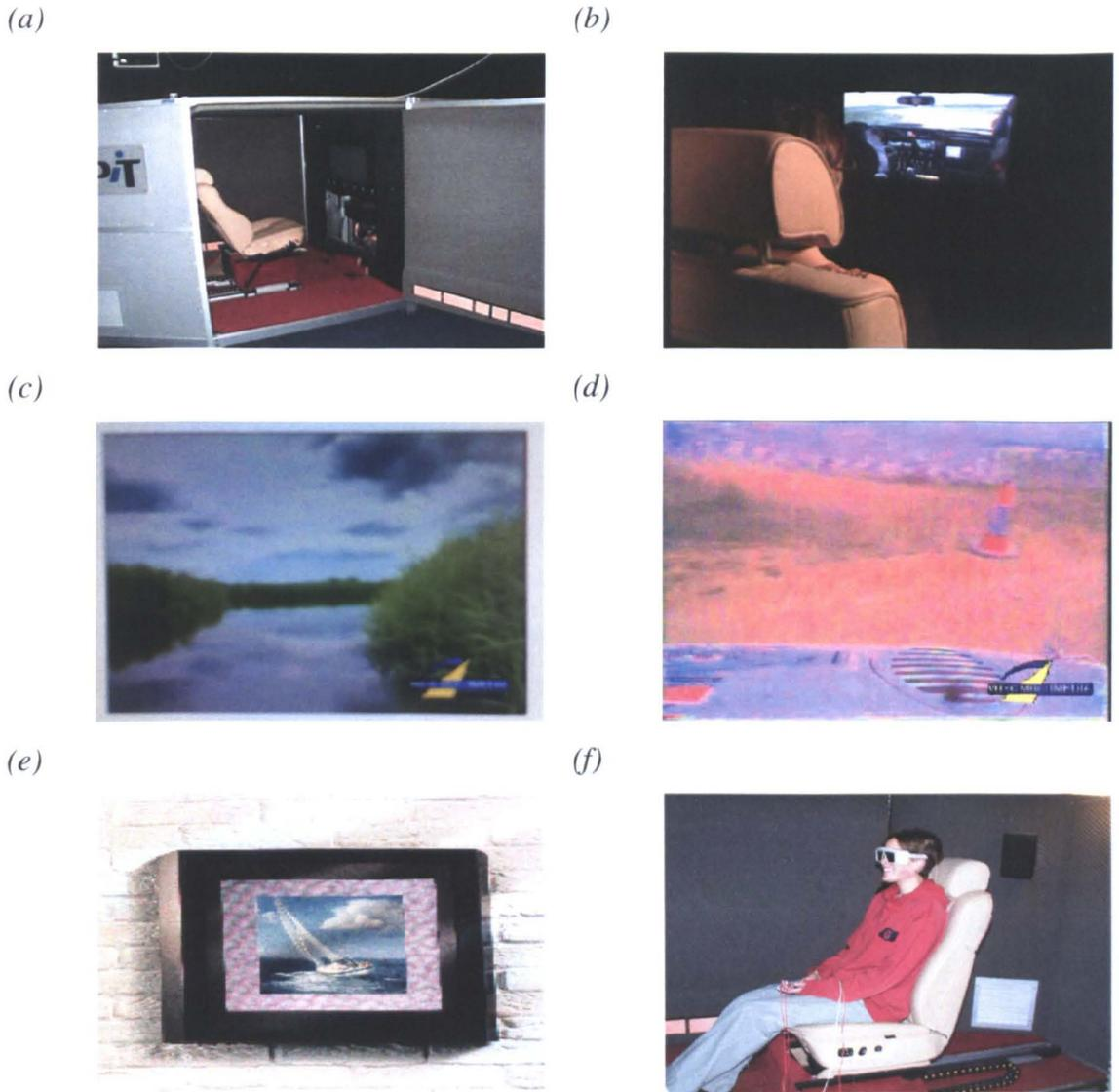
**Figure 3.1a-f** (a) The Platform for Immersive Television (PiT); (b) participant's view from the seat to the screen in the PiT; (c) a screen-shot from the BOAT video; (d) a screen-shot from the RALLY video; (e) manufacturer's marketing photograph of the Vistral screen-surround (patterned area immediately surrounding the picture of a yacht); (f) a participant seated in the PiT wearing the Crystal-Eyes spectacles and attached to the polygraph equipment.
