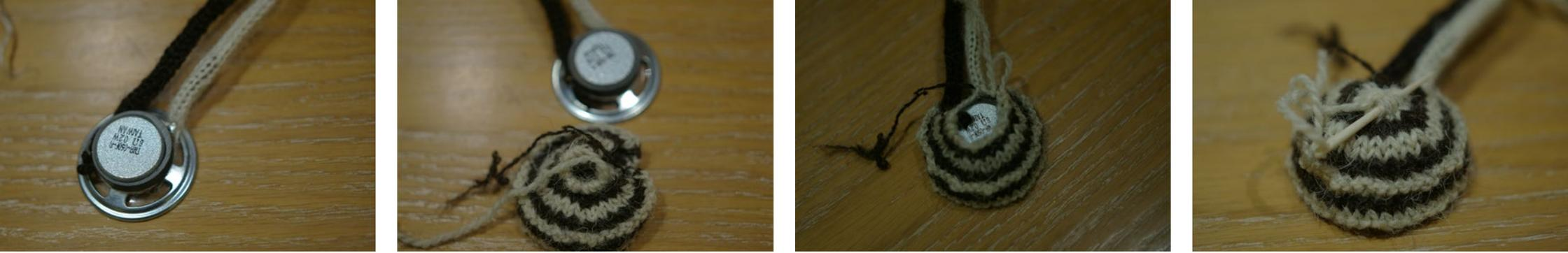
Image sequence depicting pure wool coverings being applied to speakers.
