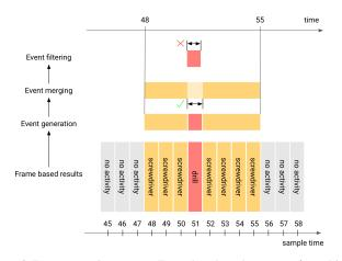
Figure 6. Event generation process. Frame-based results are transformed into events, events following each other in a close distance can be merged and very short events can be removed.
