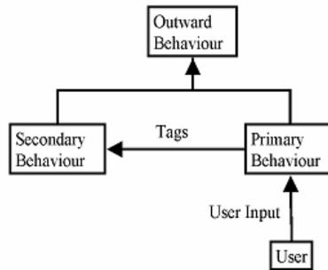
Figure 1: The relationship between primary and secondary behaviours.
