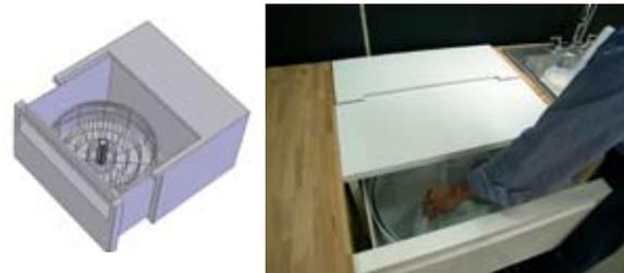
**Fig. 10e** Dishwasher: a 19" tall x 30" wide under counter pullout drawer, with lazy Susan style turntable dish rack and counter level hide-away lid. All dishes are accessible through the top lid or the drawer can be pulled out a few inches to gain further access.
