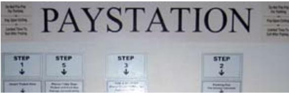
**Fig. 4** Haphazard mapping of controls during sequential interaction, like this parking garage paystation interface, is often confusing and is not considered “exploratory.” Here, additional signs attempt to cue interaction to encourage effective operation. Clear mapping of controls using the geometry of the machine and a logical reading order would support the sequence of interactivity and encourage usability.
