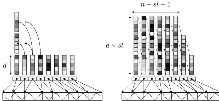
**Figure 1.** Illustration of the construction of concatenated or shingled feature vectors for our search. Note that while in principle this construction can be done for features over audio regions with temporally-varying extent and step (adjusted to the local tempo), in this paper the step size and block size were kept constant.
