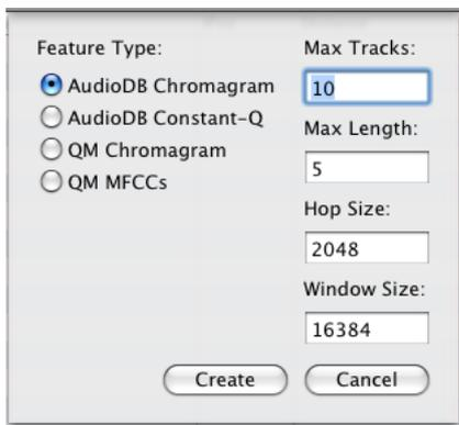
**Figure 2.** Creating a new database in iAudioDB. The feature extractor is chosen on the left-hand side, while parameters related to the database and the extractor are on the right.
