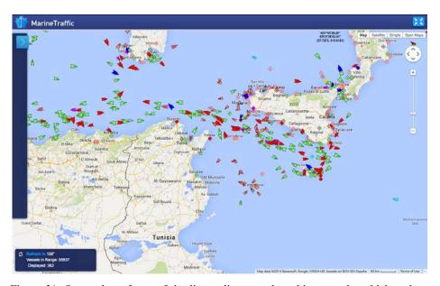
Figure 21: Screenshot of one of the live online vessel tracking portals, which gathers and presents live AIS data. Source: <a href="www.marinetraffic.com">www.marinetraffic.com</a>.
