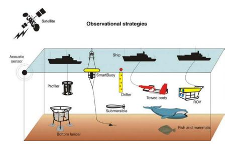
Figure 22: Schematic overview of marine observational strategies (drawing by Irene Gooch). Source: Silke Kröger and Robin J. Law, "Biosensors for Marine Applications," Biosensors and Bioelectronics, vol. 20, no. 10 (April 2005): 1905.
