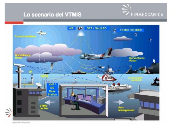
Figure 19: Finmeccanica PowerPoint slide from "Dal VTS al VT- MIS," 2007. The graphic presents the "Vessel Traffic Management and Information System" (VTMIS).
