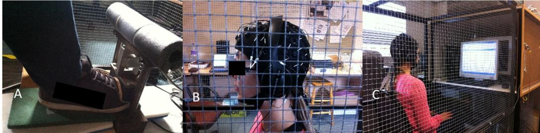
*Figure 1.* Experimental set-up of the present study. Figure 1A: Force transducer used to quantify the level of pressure generated by the participant against the load cell; Figure 1B: Participant wearing the EEG cap and headphone; Figure 1C: Participant's vision from outside the Faraday cage; the cage was assembled to prevent the electrical interference of external devices.
