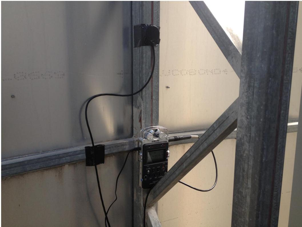
Figure 20 - Contact microphone attached to metal structure
