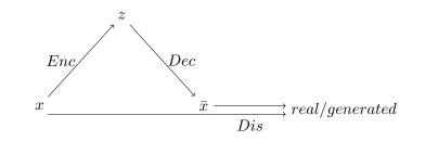
FIGURE 4.1: Overview of autoencoder model with discriminator network.
