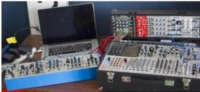
Figure 1. The Eurorack format modular synthesizer used in the case study, featuring a range of different modules including sequencers, oscillators, filters and envelope generators. Photo credit: Dom Mino.
