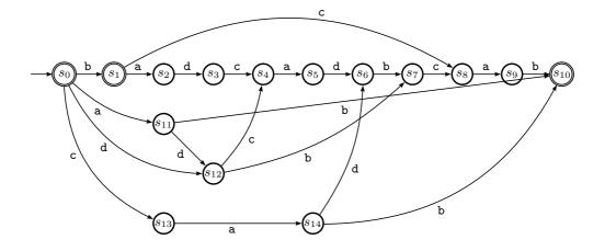
Fig. 3. Suffix automaton of string w = badcadbcab.
