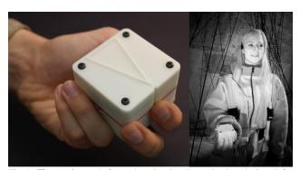
Fig 1: The 'Animotus' shape-changing haptic navigation device (left). Each audience member (right) used an Animotus to navigate the pitchblack Flatland production.
