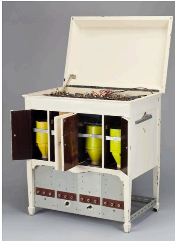
Fig. 1: Oramics wave scanners and associated circuits
