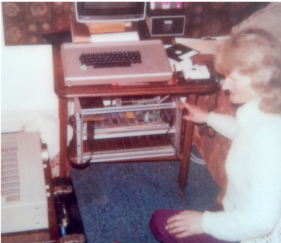
Fig 47. Oram with her Apple II computer, early 1980s. Her custom designed audio interface is clearly visible directly below the computer.
