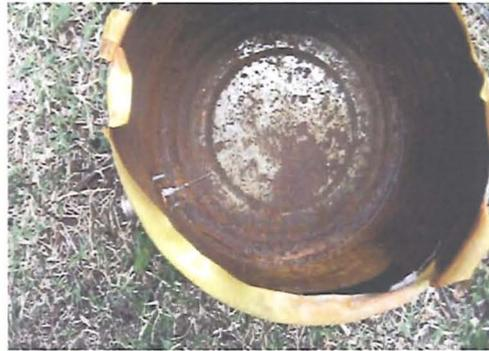
Fig. 42. Ben's home-made *cantenna* (19.11.06).
