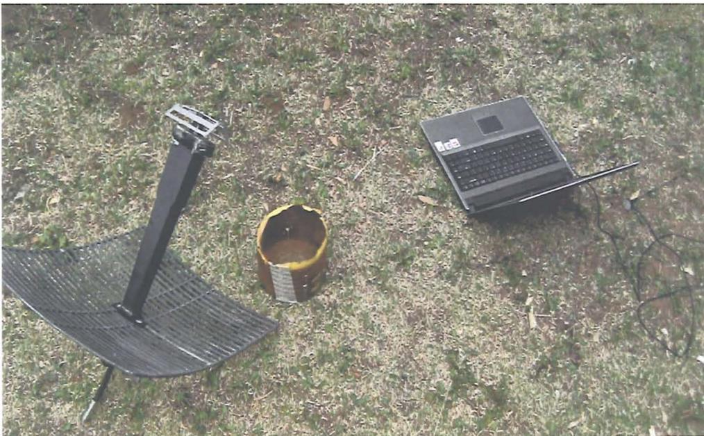
Fig. 43. Three antennas: Hills dish, *cantenna* and small magnetic car antenna (19.11.06).
