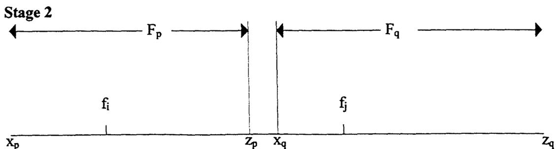
If  $C_{ij} \leq x_q - z_p$  then  $f_j - f_i \geq x_q - z_p \geq C_{ij}$  the constraint was satisfied
