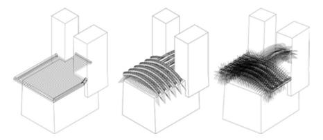
**FIGURE 6:** Three approaches to the support structure for the ceiling tested during the preparation of the 2007 technical specifications. The one on the right was chosen. Images courtesy of Arup.
