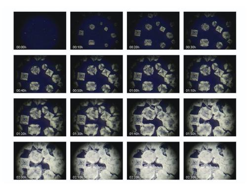
Figure 12 The formation of sea salt crystals, in my experiment at Professor Anatoly Zayats's Laboratory, at King's College London. Observed with 20x magnification reflection microscope through a polariser. Snapshots of the time-lapse recording by Mari Ohno (2018).
