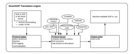
Figure 4.5: SOP translator components
