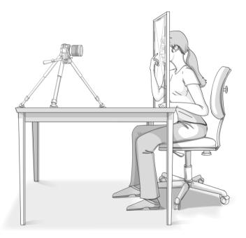
**Figure 4.14. Face localisation task.** Face apparatus and participant positioning during the face localisation task.
