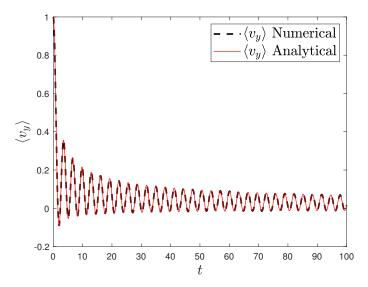
**Figure 2.** Plot of the analytical (redline) and the numerical solution of the average velocity along the *y* axis with  $\alpha = 0.5$ , T = 0.001,  $\omega_0 = \omega_1 = 1$ . Number of realizations 200k.
