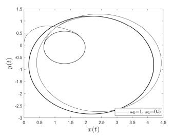
**Figure 5.** Single realization of the trajectory of a charge in the non-Poisson case. The values of the parameters are  $\alpha = 0.5$ , T = 0.001,  $\omega_0 = 1$ ,  $\omega_1 = 0.5$  and t = 500.
