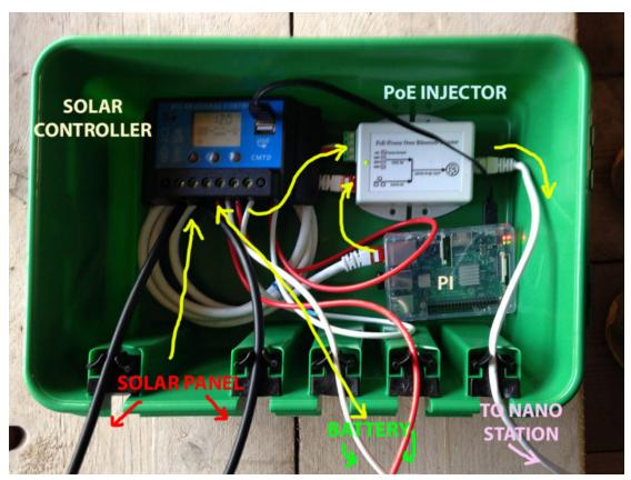
Figure 26- Part of the hardware set-up from Edge Hill Station in a waterproof box.
