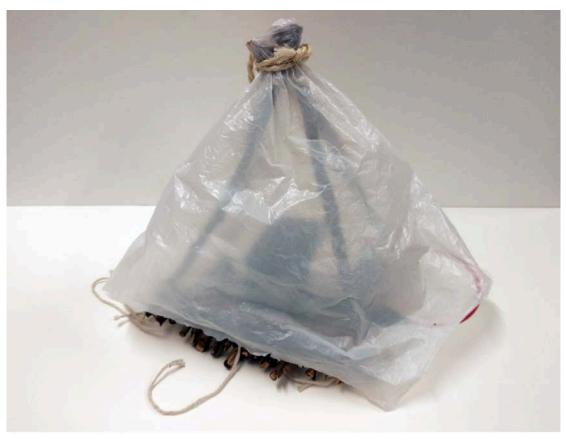
The platform, made from sticks collected from the forest floor tied together with twine. It contains a battery and Raspberry Pi 3b
