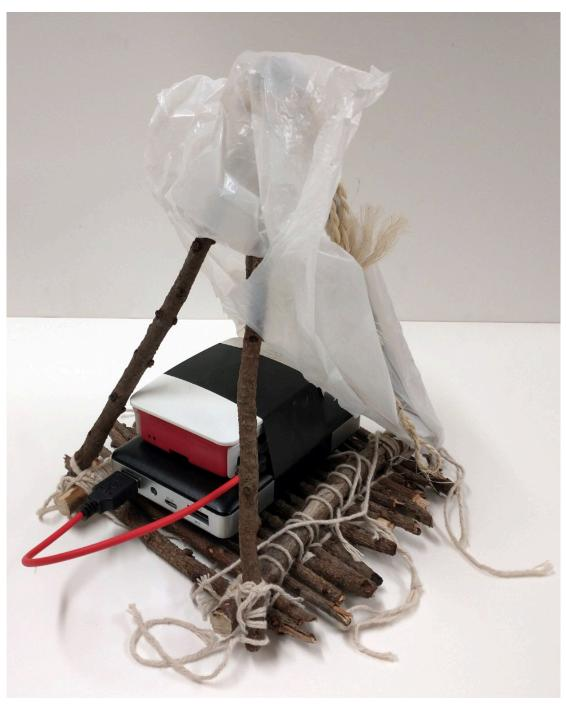
The inside of the platform that hung from the top of the mast, showing the battery and Raspberry  $\operatorname{Pi}$  3b.
