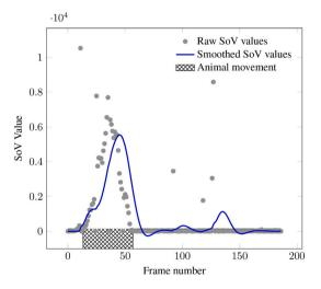
Fig. 5. Example of IIR smoothing of SoV motion filtering.
