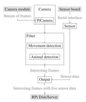
**Fig. 1.** Data flow through the system; boxes with a black outline indicate software classes/containers, whilst grey boxes represent the hardware depicted in Fig. 2.
