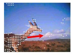
**Fig. 4.** Our SoV approach for determining motion on a video from the WCS dataset. The raw non-zero motion vectors are white, while their sum is illustrated as the large red vector. (For interpretation of the references to colour in this figure legend, the reader is referred to the web version of this article.)
