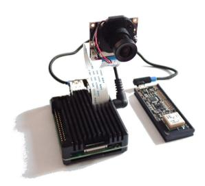
Fig. 2. RPi, camera, and DynAlkon's sensor board.
