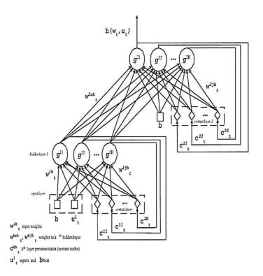
Figure 2.5: Multiple Layer Fully Connected Recurrent Artificial Neural Network: circles represent neurons, square represents the input or the bias, and the diamonds represent the context nodes.
