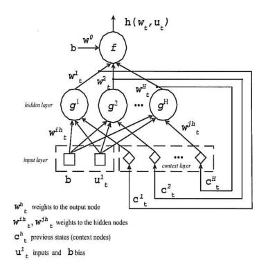
Figure 2.3: Locally Connected Recurrent Artificial Neural Network: circles represent neurons, the two squares represent the input and the bias, and the diamonds represent the context nodes
