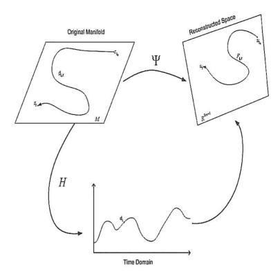
Figure 2.1: A diagram of the reconstruction framework proposed by Packard et al. [158] and proven by Takens' [203].
