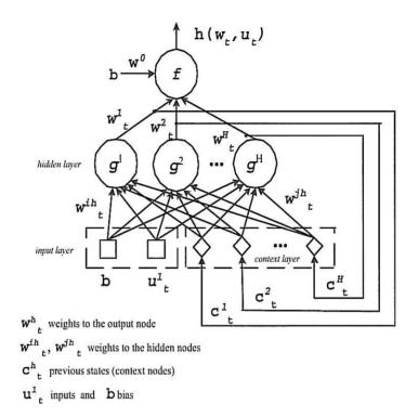
Figure 2.6: Elman Recurrent Artificial Neural Network: circles represent neurons, square represents the input and bias, and the diamonds represent the context nodes
