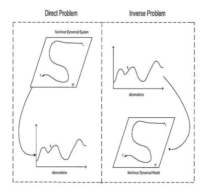
Figure 1.1: Models of dynamic systems can be built in two main ways, the Direct approach and the Inverse approach. The direct approach starts with an understanding of the underlying system. Equations of motion are written down, and the model is verified on the observables of the system. The Inverse approach starts with little or no understanding of the system. Observables of the system are used to reconstruct the equations of motion, and the model is verified on an unseen set of observables.
