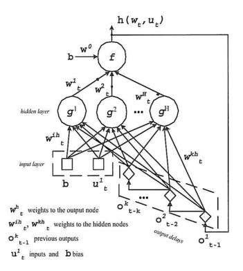
Figure 2.4: Jorden Connected Recurrent Artificial Neural Network: circles represent neurons, the two squares represent the input and bias, and the diamonds represent the context nodes
