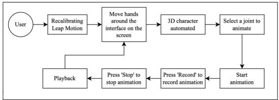
Figure 3.24: Hand gesture interface system design
