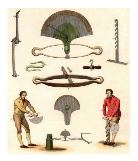
**Figure 27.**Dynamometer, an instrument for measuring mechanical force or power, designed by Edme Regnier. Engraving from *Encyclopaedia Londinensis* (London, 1803). Digital image courtesy of World History Archive / Alamy Stock Photo (all rights reserved).
