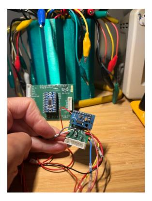
Figure 49 The circuit board in each bot.
