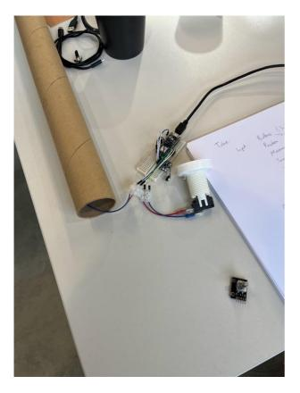
Figure 71 Completed Rough Prototype including button installed in the top of a cardboard tube and circuit board with haptics attached.
