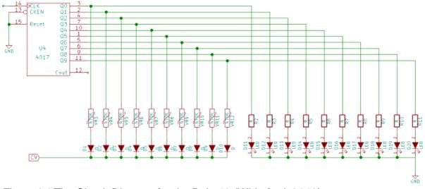
Figure 24 The Circuit Diagram for the Baby10 (Whiteford, 2016)
