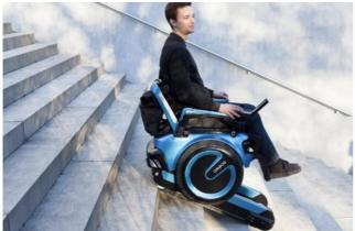
Figure 9 The scewo is a self-balancing wheelchair that can go up and down stairs. (designboom, 2017)
