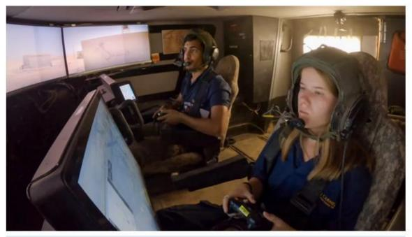
Figure 2 IAI staff use the Carmel's Xbox controller interface to control the prototype armoured fighting vehicle. (Courtesy of Israel Aerospace Industries)(Smith, 2022)
