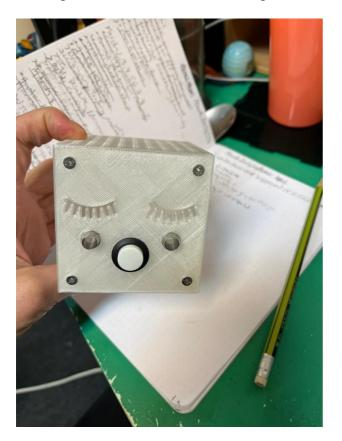
Figure 69 Improved casing for version 4 showing inset screws.
