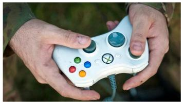
Figure 1 U.S. Army Spc. Andrew B. Clement, an explosive ordnance disposal technician from Jackson, Tenn., assigned to 129th EOD, attached to 3rd Brigade Combat Team, 25th Infantry Division, Task Force Bronco, uses an Xbox controller to operate an EOD robot at Combat Outpost Honaker-Miracle in eastern Afghanistan's Kunar province, Aug. 1, 2011. (U.S. Army photo/Sgt. 1st Class Mark Burrell).("The US military will fight the next big war with Xbox-style video game controllers," 2023)
