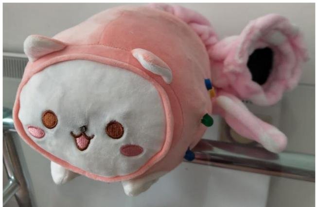
Figure 79 The cat synth, SYNTHia showing the buttons, speaker and sensors embedded in the cat plushie.
