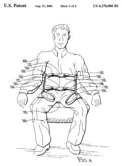
Figure 8 An illustration from a 1999 patent application showing a Tyvek harness for lifting passengers from an onboard wheelchair into their seat. Sling for transporting a person into a chair and method of using the same invented by Judy Hoit, US Patent 6276006B (Hickman, 2020)
