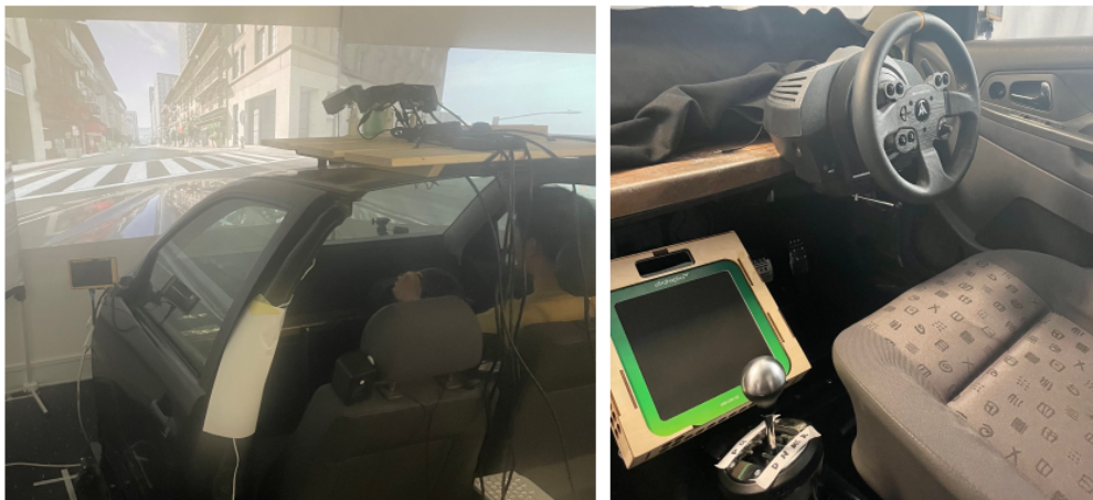
Figure 2: Driving simulator setup, internal and external.
