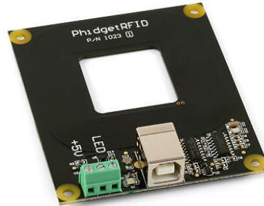
Figure 3 Phidget RFID reader
