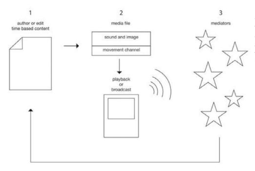
Fig. 6 A time-coded text file is embedded in a QuickTime movie; this broadcasts control messages via a USB peripheral as the movie plays. A demo can be seen at http://www. tobiekerridge.co.uk/mm/mov/11\_ livedemo.mov.
