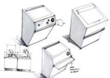
Fig. 10f Laundry: 30" wide units at counter depth with wide diameter shallow drums to promote easy reach and access through larger front-loading doors. Configured to break the counter line to place doors at optimal height to limit bending and stooping.
