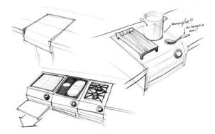
**Fig. 10c** Cook Top: a flexible system that enables multiple configurations of induction, electric and gas units. These units would be located flush to counter surface to enable a user to slide pots off the cooking surface to the counter thereby eliminating excessive reaching and lifting of heavy, hot cookware.
