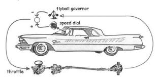
Figure 7 Feedback system (cruise control)..
