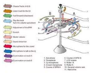
**Figure 3** Saturn sound mixer functional scheme
