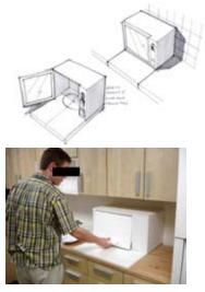
**Fig. 10d** Microwave: a slide-in unit into the counter surface where the turntable is at counter line enabling arthritic hands to slide hot dishes and liquids safely from within the microwave to the counter surface.
