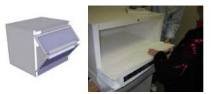
Fig. 10b Wall Oven: a split folding door enables hot surfaces to mate and minimize reach-over length. This can reduce accidental burns and would provide a surface at counter line to slide out hot cookware.
