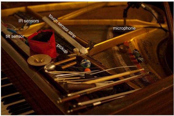
Figure A14: *piano*+ preparations, tools and sensors The sensors are connected to the gluion board sending the sensor data as OSC via the ethernet connection to Max. (photo © Sebastian Lexer 2010)
