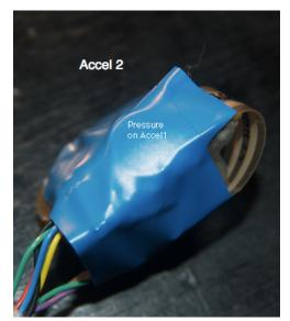
Figure A16: tilt sensor Accel 2 with an additional pressure sensor
