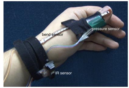
Figure B9: experimental 'glove' with distance, bend and pressure sensors
