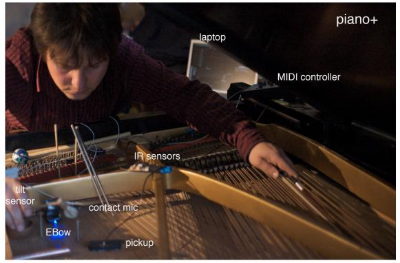
Figure A13: *piano*+ preparations, tools, sensors, contact microphone and pickup (photo © Elke Schwarz 2010)
