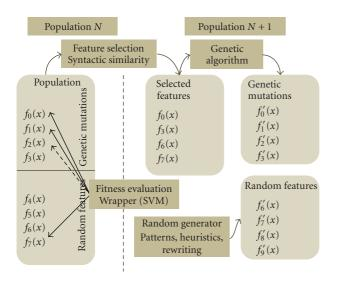
FIGURE 3: The architecture of AF generation. AFs are evaluated individually using a wrapper approach. AFs are selected for the next population using a syntactic feature selection algorithm.
