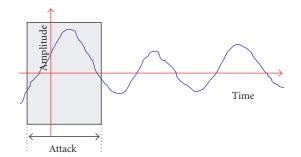
FIGURE 8: A full sound and its attack portion. The attack is defined by an amplitude threshold: when the amplitude goes above the threshold, the attack begins, and when it eventually goes under, the attack ends. In practice, we consider 128 samples after the beginning of the attack, that is, about 3 milliseconds.
