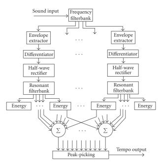
FIGURE 2: The tempo extractor from Scheirer [52] is a typical example of a high-level audio feature.
