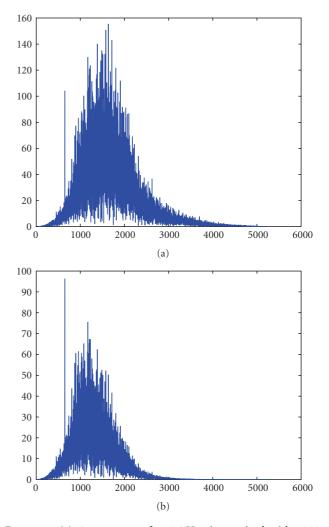
FIGURE 4: (a) A spectrum of a 650 Hz sinus mixed with 1000–2000 Hz colored noise. (b) A spectrum of a 650 Hz sinus mixed with 1000–2000 Hz colored noise, prefiltered by a 1000 Hz low-pass filter.
