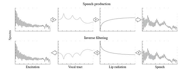
Figure 2.1: Inverse filtering: the upper row represents the separated speech production model; the lower row illustrates the corresponding inverse filtering process, in which the lip radiation and vocal tract filters are inverted to acquire an estimate for the glottal flow waveform (reproduced from Airas 2008, p. 50, with permission by Informa Group)
