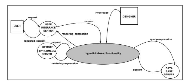
Figure 1: A General, Open Architecture for Hypermedia Systems
