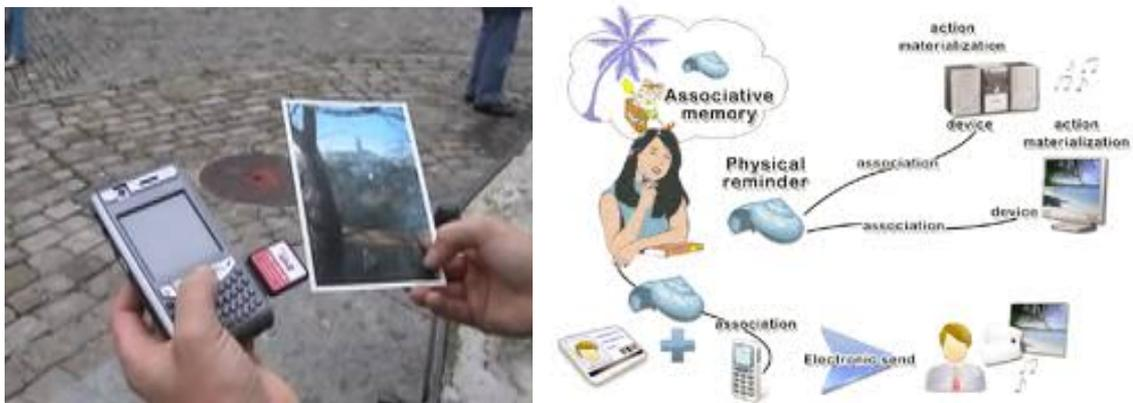
Figure 20: Memodules, by Mugellini et al. (2007), are small tagged physical objects that form a link to multimedia information that can be accessed by several devices.
