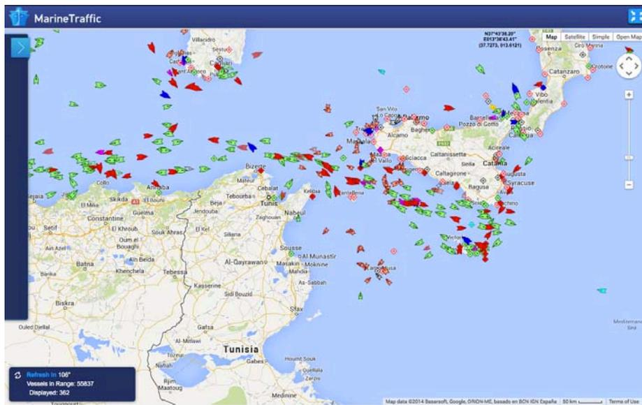
Figure 21: Screenshot of one of the live online vessel tracking portals, which gathers and presents live AIS data. Source: [www.marinetraffic.com](http://www.marinetraffic.com).
