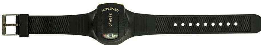
*Figure 4.1.* GENEActiv accelerometer device used for INMI tempo measurements.
