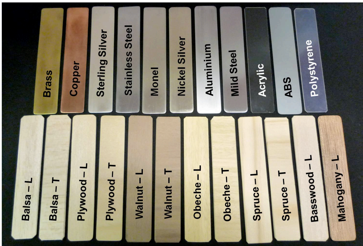
Fig. 2. A picture of the 23 materials samples used in this study, made from metals, woods and polymers.
