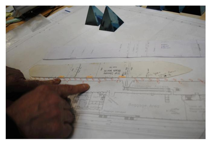
We start our 'tour' inside the office, "where it all begins". John [fake name] shows me the drawings they use to plan the operations in the terminals, adjusting the yokohamas (movable pneumatic ship fenders) and gangways to the design of each particular ship (or family of ships – since some from the same company have similar technical characteristics). [Fieldnotes, Dover, 3<sup>rd</sup> April 2012]
