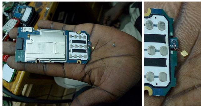
**Figure 2: The discarded microphone is visible on Jason's palm. He has connected a replacement microphone using four copper wires, rather than mounting it on the motherboard, as can be seen in the magnified image, September, 2012.**
