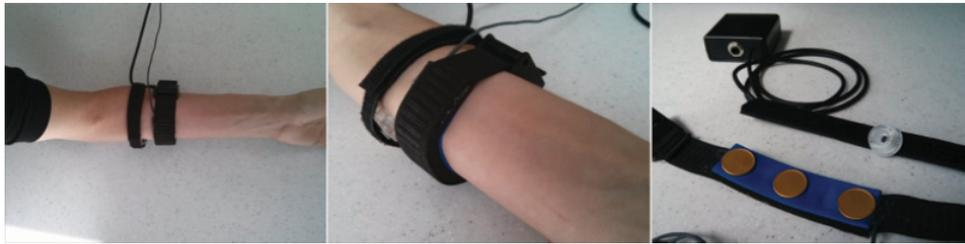
Fig. 3. Experimental setup. Left: EMG and MMG sensors placed on the forearm. Middle: EMG and MMG sensors placed on the forearm (close view). Right: The EMG (left) and MMG (right) sensors.
