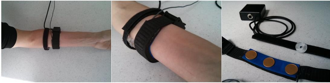
Figure 6.4: The sensor setup used in the third part of the experiment on gesture expressivity. Pictured are both the biosensors we used to capture MMG and EMG from arm gesture. The rightmost image shows the XTH Sense, at the top, and the Bioflex, at the bottom.
