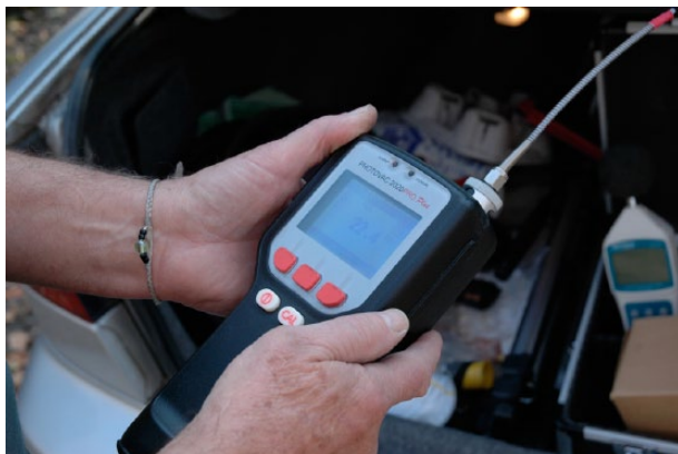
Figure 2. Citizen monitoring VOCs near compressor station in northeastern Pennsylvania. Citizen Sense 2013.
