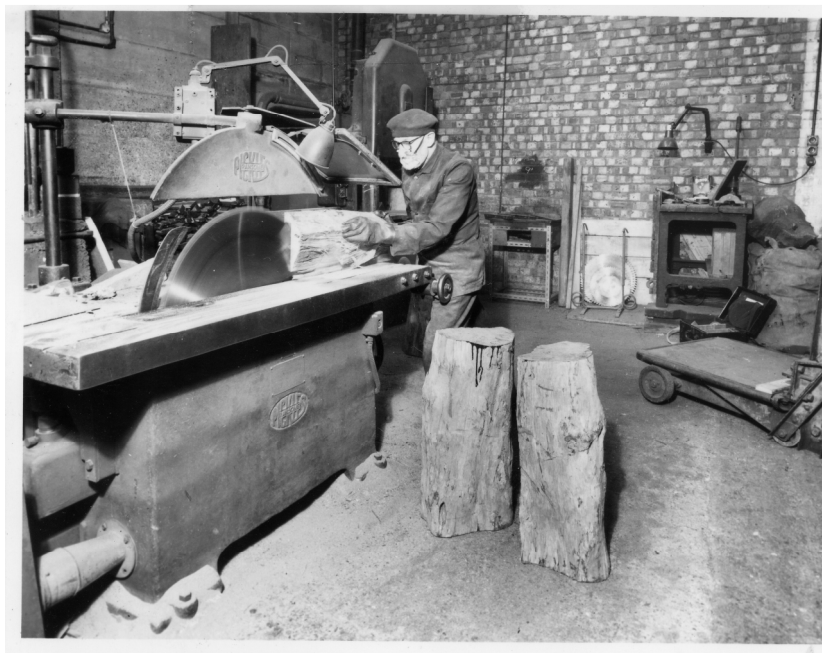
Figure 1-7 A Boosey & Hawkes workman protects himself from the toxic dust produced when sawing African blackwood.
