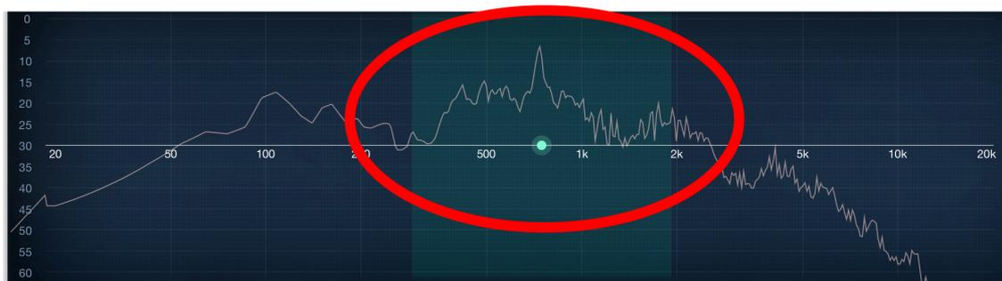
**Figure 8.15.** The frequency response of the sound recording of a car engine shows the 750Hz as the highest amplitude frequency.
