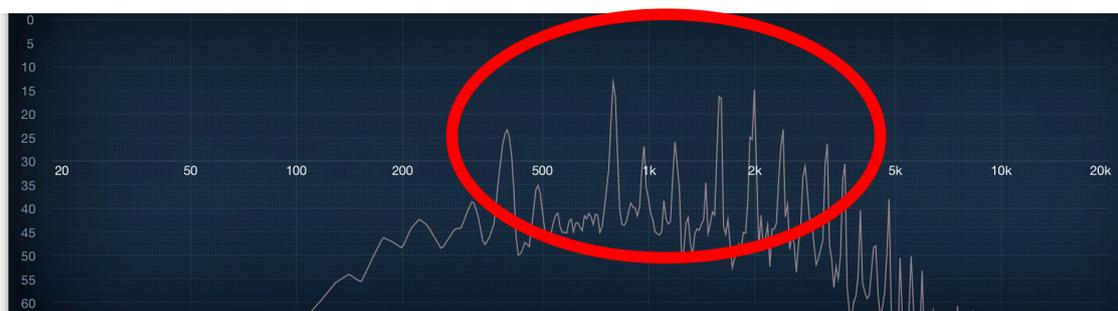
**Figure 8.13.** Frequency response of a French horn single note.
