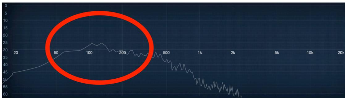
**Figure 8.19.** Frequency response of the audio recording of the wind.
