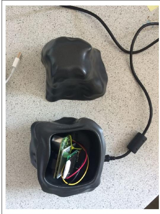
**Figure 3.** Dustbox particulate matter 2.5 monitor.
