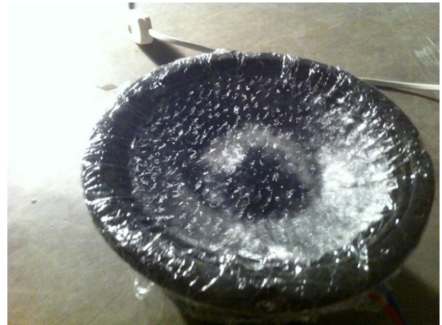
Fig. 3: Water vibrating in one of the speaker cones of the larger prototype
