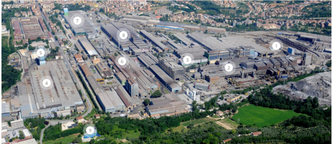
Figure 9. (1) scrap yard; (2) malting shop; (3) slab continuous casting; (4) PIX 1 cold rolling; (5) bright annealing; (6) forging division; (7) PIX 2 cold rolling; (8) hot rolling mill; (9) IT service (source: http://www.acciaiterni.it/en/about-us/plants/ )
