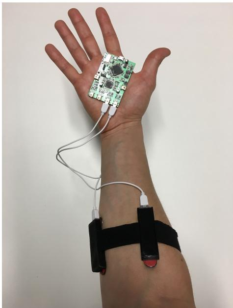
Figure 1: Board prototype worn on right forearm.
