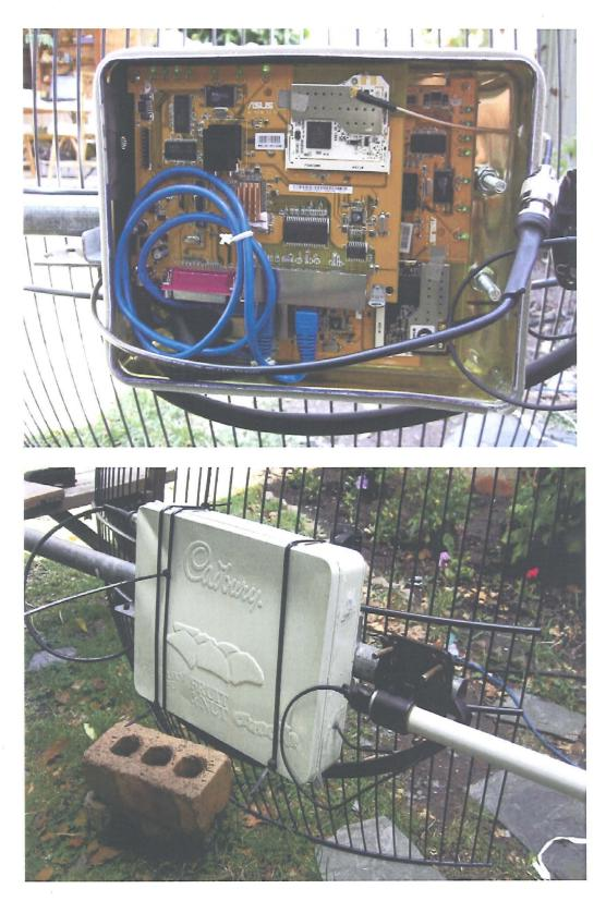
Fig. 33. Inside and outside the biscuit tin node box (13.11.06).
