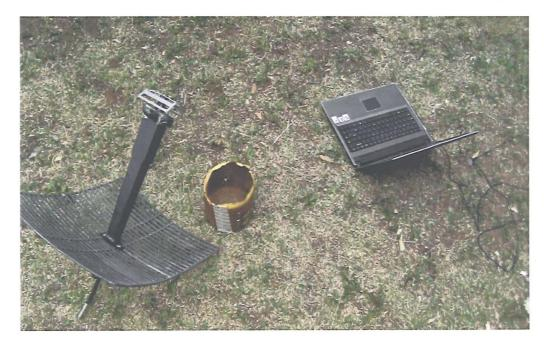
Fig. 43. Three antennas; Hills dish, cantenna and small magnetic car antenna (19.11.06).
